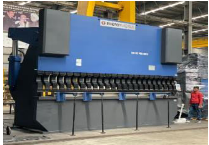
Press Brake Rear Cylinder (500 Ton X 5 m)
